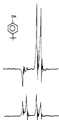
Figure 4. ^1\text{H} NMR spectra (60 MHz) of a solution of 0.1 M 4- tert -butylphenol and 0.1 M decadeuteriobenzophenone in benzene- d_6 in the dark (bottom) and during UV irradiation (top).
